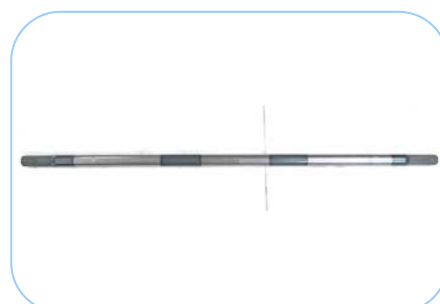
Middle Shaft M5000 ,Front 16T x 16T W 24 mm. Long 890 mm.
