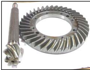
Crown Wheel + Pinion ( Rear ) L3408, 37T
