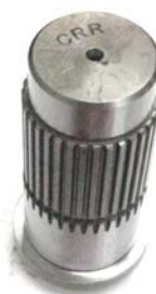
Front Wheel Hub Shaft M5000 34T
