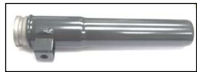
Pipe, Middle Shaft L4508-L4708 (Rear-Short) Long: 210 x Hole: 30.50/ 31.50 x Out: 35/38 mm
