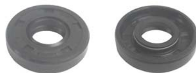
Seal, Drive Shaft Gear, L3408 AE1052E Inside 20.50 x out side 47.25 x high 10 mm.
