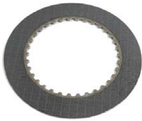
Clutch Plate PTO. M5000 34T Inside 60.50 x Outside 89.75 x Thickness 1.80 mm
