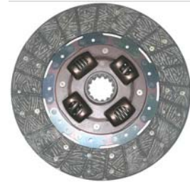
Clutch Plate M5000 11" x 14T CODE : 6-05-100-07 3A272-25130
