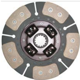
Clutch Plate M7040 11" x 14T CODE : 6-05-100-08 3A261-25130
