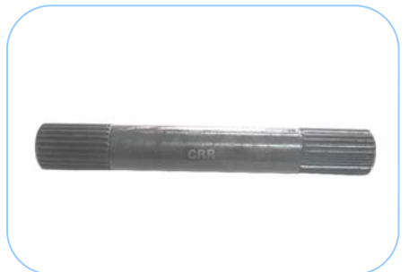
Steering Shaft L3408 24Tx24T CODE : 5-01-208-14 L 174 mm. W. 23.75 mm. TC402-12720
