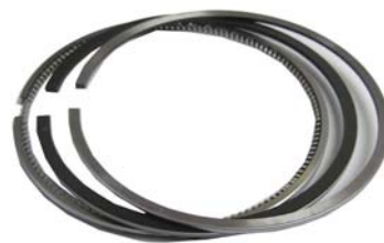
Piston Ring Set M9000, M8200, 98 mm.
