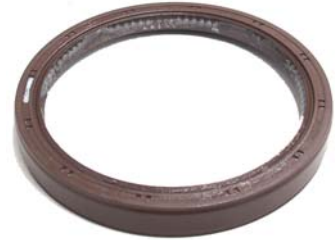
Housing Seal, Rear (Brown) EF453T BH1517I In:83.50*Out: 102* H:12mm CODE: 5-08-200-36 129648-01780
