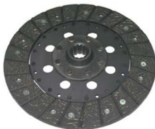
Clutch Plate EF 352 T 9" X 13T CODE : 6-05-100-05 198287-21510
